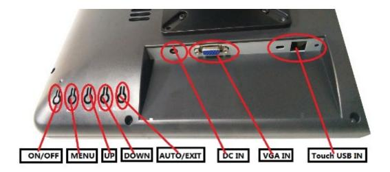
TOUCH USB: this is connected to PC's USB Ports; used for touch function DC in: 12V DC in; power supply for the touch monitor VGA in: this is connected to PC's VGA output port
